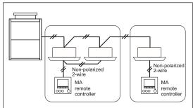
\*When a PAR-33MAA(G) is connected to a group, no other MA remote controllers can be connected to the same group.
