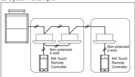
\*When a PAR-CT01MAU is connected to a group, no other MA remote controllers can be connected to the same group.
