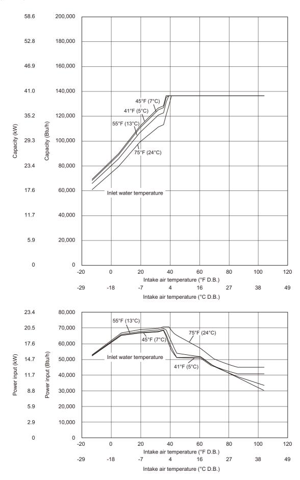
Outlet water temperature 130°F (54°C) Max capacity operation mode
