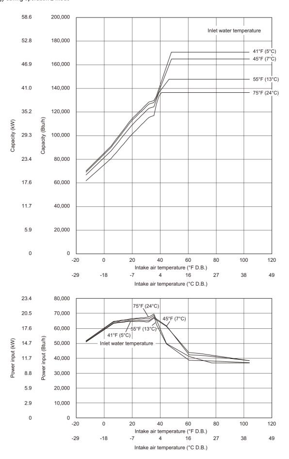
Outlet water temperature 170°F (77°C) Energy saving operation 2 mode
