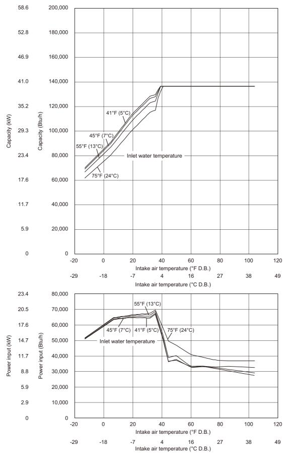
Outlet water temperature 150°F (66°C) Energy saving operation 1 mode
