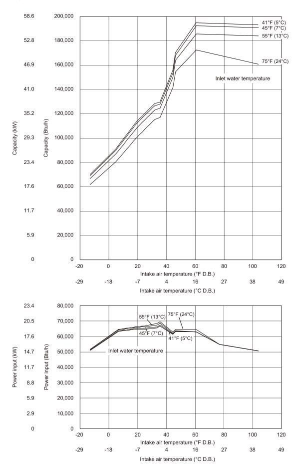
Outlet water temperature 170°F (77°C) Max capacity operation mode
