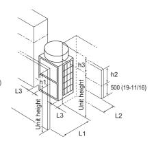
Add the dimension that exceeds the height limit (shown as "h1" through "h3" in the figures) to L1, L2, and L3 as shown in the table below.
