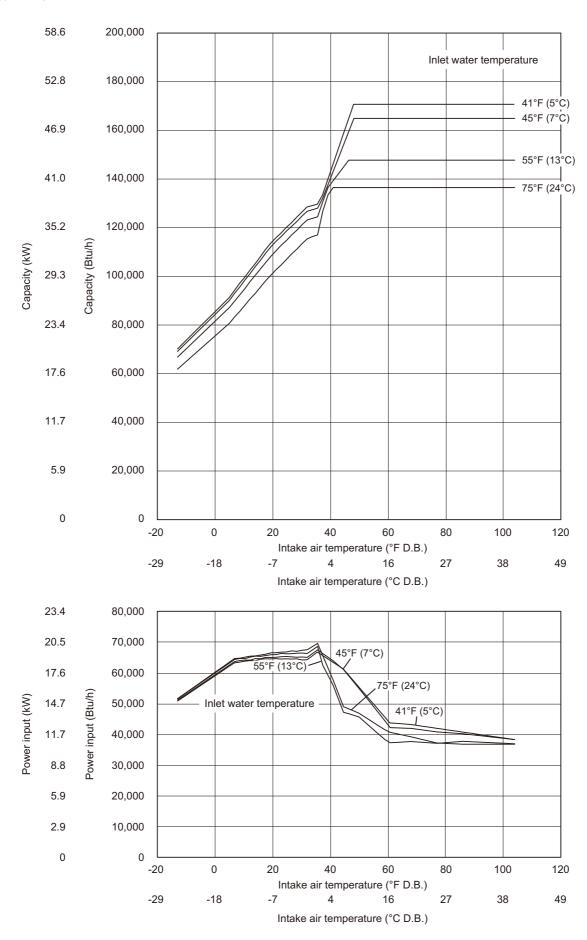
Outlet water temperature 150°F (66°C) Energy saving operation 2 mode
