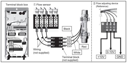
Connect the flow sensor wiring to the terminal block inside the BOX. The numbers on the wirings correspond to the numbers on the terminal block
