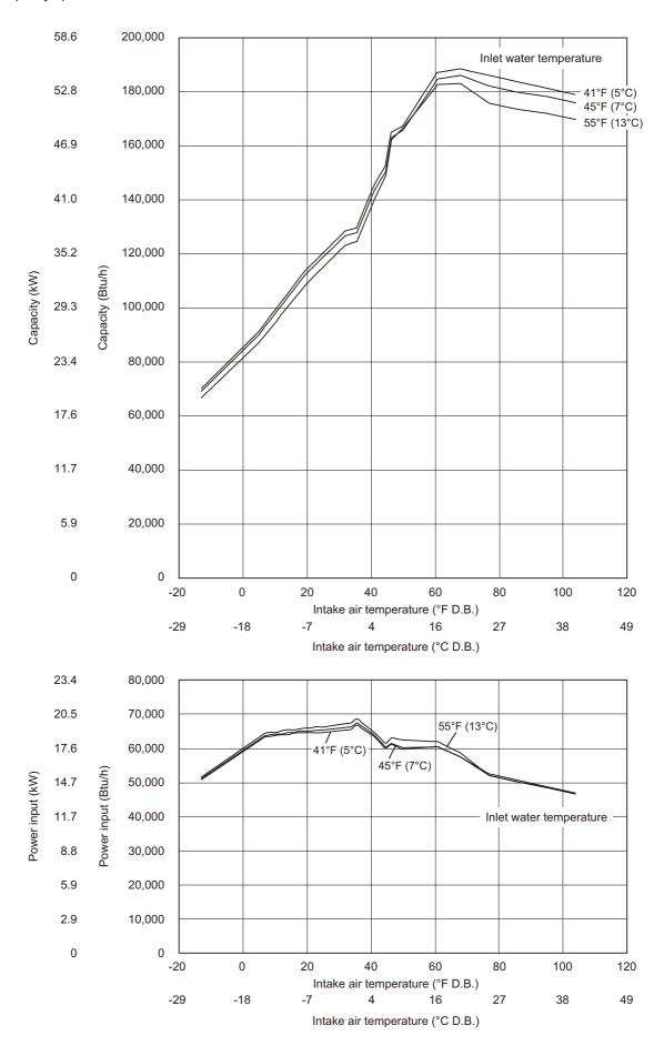
Outlet water temperature 150°F (66°C) Max capacity operation mode
