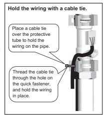
Insert the flow sensor into the couplers, and then fit the quick fasteners where the flow sensor and the couplers are connected to each other. Keep the quick fasteners out of contact with the wiring so as not to damage the wiring. Hold the wiring to the quick fastener with a (short) cable tie as shown in the figure to keep the wiring from being damaged.
