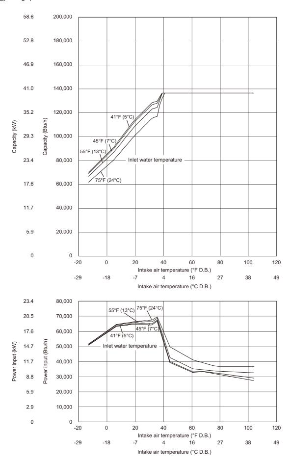
Outlet water temperature 170°F (77°C) Energy saving operation 1 mode
