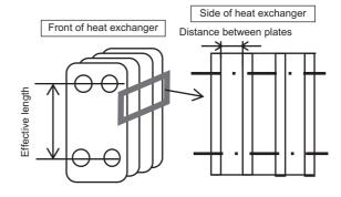
A shearing stress of 16 Pa (0.01 ftAq) or higher is required to reduce the amount of scale that adheres. If the shearing stress is low:
