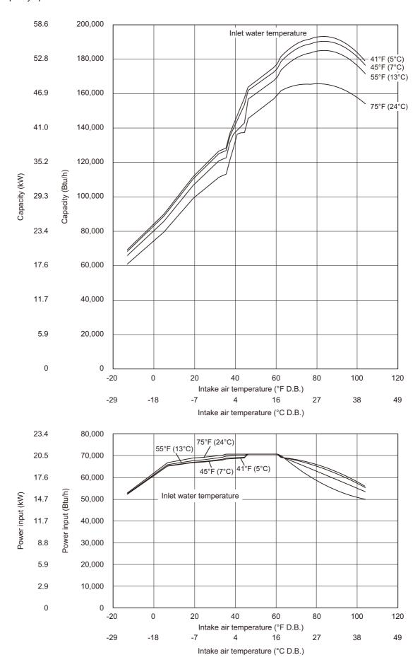
Outlet water temperature 130°F (54°C) Energy saving operation 2 mode
