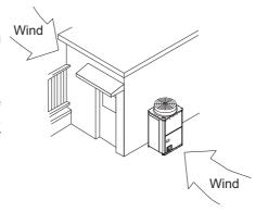
Install the outdoor unit in a place where it is not exposed to direct wind, such as behind a building.
