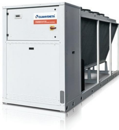
**Air-Source Heat Pumps for outdoor installation, for the production of chilled or hot water. The units feature hermetic scroll compressors using R-410A refrigerant, axial fans, plate heat exchanger, condensing coils with copper tubes and aluminum fins and electronic expansion valve. The range is composed by units equipped with two compressors in a single-circuit configuration.**
