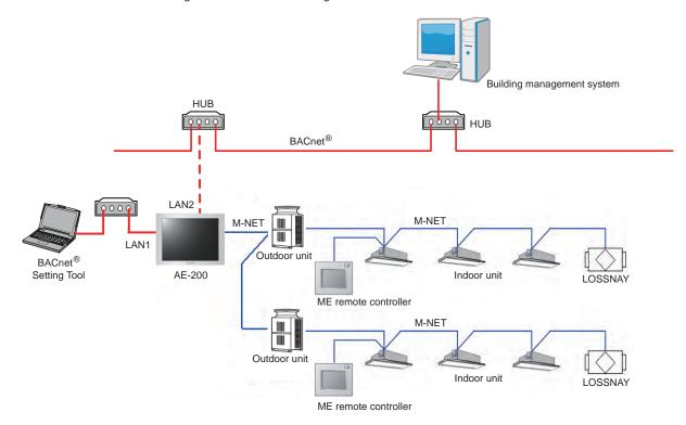
Before performing BACnet<sup>®</sup> settings for the AE-200 using the BACnet<sup>®</sup> Setting Tool, it is necessary to set indoor unit group settings on the AE-200 Initial Setting Tool. Refer to section 5-4 "Initial setting procedure" for details. For systems that use multiple AE-200, set all AE-200 connected to BACnet<sup>®</sup> individually using the BACnet<sup>®</sup> Setting Tool.
