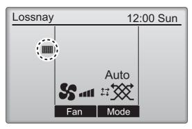
will appear on the Main display when it is time to clean the filter and/or Lossnay core.
