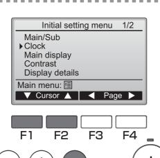
Move the cursor to the "Clock" with the F1 or F2 button, and press the SELECT button.
