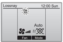
will appear on the Main display when the weekly timer setting for the current day exists. The icon will not appear while the On/Off timer is enabled or the system is under centralized control (Timer operation from local remote controller is prohibited).
