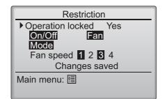
The screen to make the settings for the operation lock function will appear.
