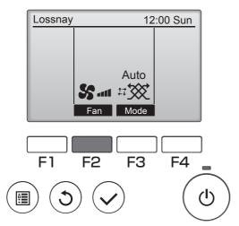
Press the F2 button to go through the fan speeds in the following order.
