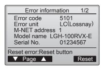
Error code, error unit, M-NET address, unit model name, and serial number will appear. The model name and serial number will appear only if the information have been registered.
