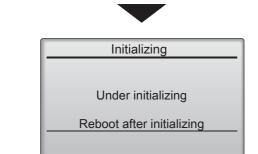
After initialization is executed, the remote controller reboots automatically.
