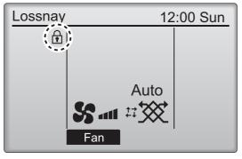
will appear on the Main display when the operation lock function setting is enabled.
