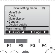
Move the cursor to the "Contrast" with the F1 or F2 button, and press the SELECT button.
