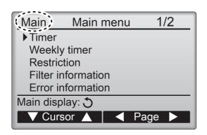
The following settings cannot be made from the sub remote controller. Make these settings from the main remote controller. "Main" is displayed in the title of the Main
