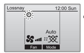
will appear on the Main display when the On/Off timer is enabled.
