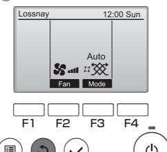
Press the RETURN button to exit the Main menu and return to the Main display.
