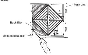
3. Hold the handle and draw the Lossnay cores out from the main unit
