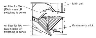
Remove the back filters from the main unit with the maintenance stick
