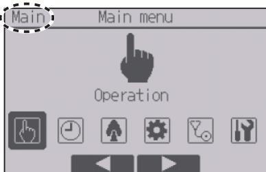
The following settings cannot be made from the sub remote controller. Make these settings from the main remote controller. "Main" is displayed in the title of the Main menu on the main remote controller.
