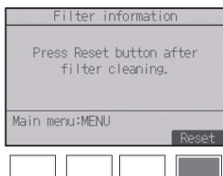
Press the **F4** button to reset filter sign.
