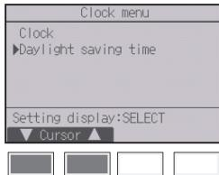
Move the cursor to "Daylight saving time" with the [F1] or [F2] button, and press the [SELECT/HOLD] button.
