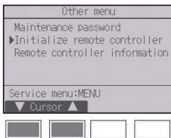
Move the cursor to "Initialize remote controller" with the **F1** or **F2** button, and press the **SELECT/HOLD** button.
