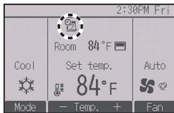
will appear on the Main display in the Full mode when the weekly timer setting for the current day exists.
