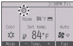
will appear on the Main display in the Full mode when the Auto-Off timer is enabled. The icon will not appear while the HOLD function is enabled.
