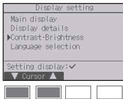
Move the cursor to “Contrast•Brightness” with the [F1] or [F2] button, and press the [SELECT/HOLD] button.
