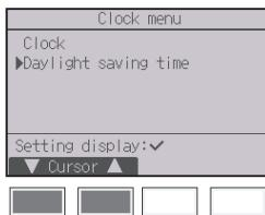
Move the cursor to "Daylight saving time" with the [F1] or [F2] button, and press the [SELECT/HOLD] button.
