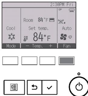
Each pressing of the **F4** button cycles through the following fan speeds.
