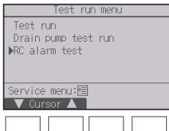
Select "RC alarm test" from the Test run menu, and press the [SELECT/HOLD] button.
