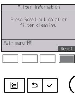
Press the [F4] button to reset filter sign.
