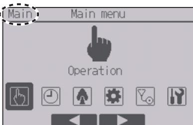
The following settings cannot be made from the supervisor remote controller. Make these settings from the main remote controller. "Main" is displayed in the title of the Main menu on the main remote controller.
