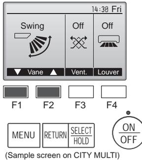
Press the [F1] or [F2] button to go through the vane setting options: "Auto", "Step 1", "Step 2", "Step 3", "Step 4", "Step 5" and "Swing". Select the desired setting.
