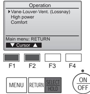
Select "Vane-Louver-Vent. (Lossnay)" from the Operation menu, and press the [SELECT/HOLD] button.
