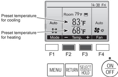
① The current preset temperatures will appear. Press the [F2] or [F3] button to display the setting screen.
