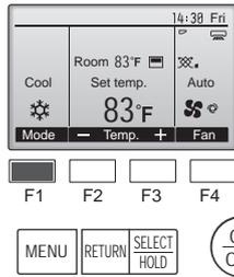
Each pressing of the [F1] button cycles through the following operation modes. Select the desired operation mode.
