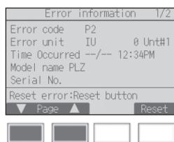
Error code, error unit, refrigerant address, unit model name, and serial number will appear. The model name and serial number will appear only if the information has been registered.
