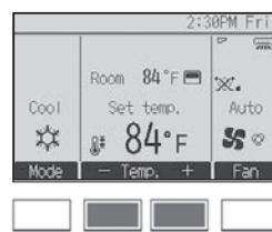
Press the [F2] button to decrease the set temperature, and press the [F3] button to increase.
