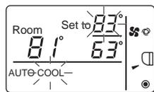
While the cooling preset temperature display blinks, pressing the **TEMP.▲** button increases the cooling preset temperature, and pressing the **TEMP.▼** button decreases the cooling preset temperature.
