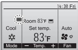
The filter sign icon will appear on the Main display in the Full mode when it is time to clean the filters.
