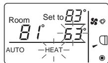
While the heating preset temperature display blinks, pressing the **TEMP.▲** button increases the heating preset temperature, and pressing the **TEMP.▼** button decreases the heating preset temperature.
