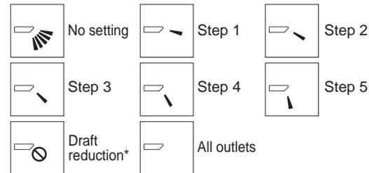
Press the [SELECT/HOLD] button to save the settings. A screen will appear that indicates the setting information is being transmitted. The setting changes will be made to the selected outlet. The screen will automatically return to the one shown above (step 5) when the transmission is completed. Make the settings for other outlets, following the same procedures.
