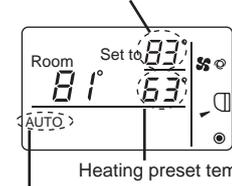
Current preset temperature (cooling/heating) appears.
