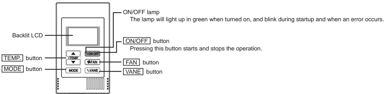
\* To set the functions that are not available on this controller (PAC-YT53CRAU) such as Louver, use MA remote controller or the centralized controller.
