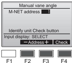
③ Select the "M-NET address" for the units to whose vanes are to be fixed, with the [F2] or [F3] button, and press the [SELECT/HOLD] button. Press the [F4] button to confirm the unit. The vane of only the target indoor unit is pointing downward.
