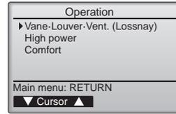
Select "Vane-Louver-Vent. (Lossnay)" from the Operation menu, and press the [SELECT/HOLD] button.
