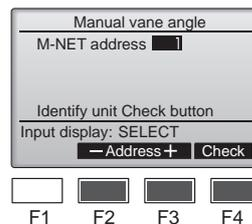
① Select the "M-NET address" for the units to whose vanes are to be fixed, with the [F2] or [F3] button. Press the [F4] button to confirm the unit.
