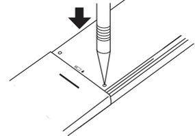
Press the Reset button with an object that has a narrow end.
