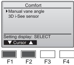
② Select "Manual vane angle" with the [F1] or [F2] button, and press the [SELECT/HOLD] button.
