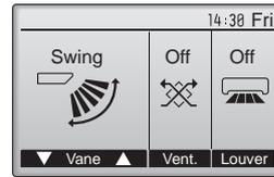
Press the [F1] or [F2] button to go through the vane setting options: "Auto", "Step 1", "Step 2", "Step 3", "Step 4", "Step 5" and "Swing".
