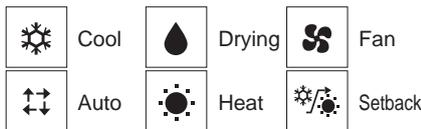
• Operation modes that are not available to the connected outdoor unit models will not appear on the display.
