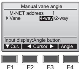
④ Select "Vane" with the [F1] button. Select "4-way" or "2-way" with the [F2] or [F3] button, and press the [F4] button.
