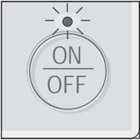
Press the [ON/OFF] button. The ON/OFF lamp will light up in green, and the operation will start. When "LED lighting" is set to "No", the ON/OFF lamp will not light up.
