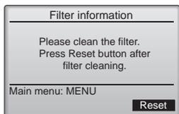
Press the [F4] button to reset filter sign. Refer to the indoor unit Instructions Manual for how to clean the filter.
