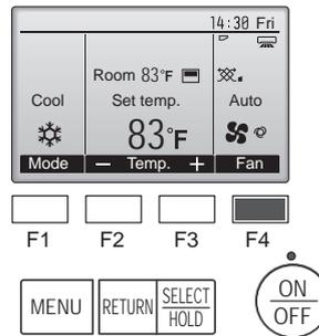
Each pressing of the [F4] button cycles through the following fan speeds.
