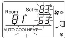
While the preset temperature (cooling/heating) display blinks, pressing the **TEMP.▲** button increases the preset temperatures for both cooling and heating, and pressing the **TEMP.▼** button decreases the preset temperatures for both cooling and heating.
