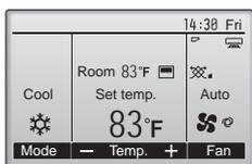
Each pressing of the [F1] button cycles through the following operation modes. Select the desired operation mode.
