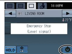
Displays ON/OFF level-signal input
