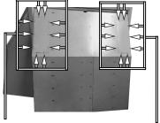
I. Install the each of the RE Access Doors with the supplied #8 HWH Screws to the RE RHS Front Panel & RE LHS Front Panel using the provided holes.
