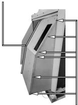
E. With the supplied #8 HWH Screws attach the RE RHS Panel to the RE RHS Front using the provide holes.
