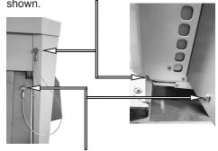
H.2. Tighten the (2) screws already installed on the Snow Guard.
