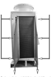
A. Install the SD RHS Panel as shown using the existing (3) SCREWS while keeping the side wire grille in place (Please Note: The SD RHS Panels are to be installed between the cabinet and side wire grille).
