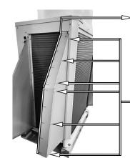
D. Install the ½" Wide Anti-Vibration Foam on to the exterior leftside edge of the SD RHS Front Panel as shown.
