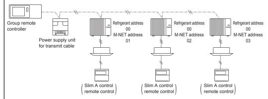
Between the outdoor units, it is OK that only M-NET wiring (2 wires, no polarity) is done.
