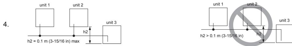
The NG example shows that oil accumulates into unit 3 while unit 1 is in operation, and unit 3 is stopped. Difference between unit and unit in height (h2) should be 0.1 m (3-15/16 in) or below.
