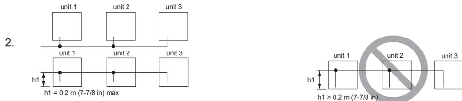
The NG example shows that oil accumulates into units 1 and 2 while unit 3 is in operation, and units 1 and 2 are stopped. Vertical pipe height (h1) should be 0.2 m (7-7/8 in) or below.
