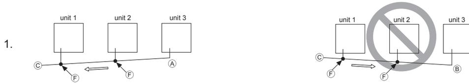
The NG example shows that oil accumulates because the units are installed on a reverse gradient while unit 1 is in operation, and unit 3 is stopped.
