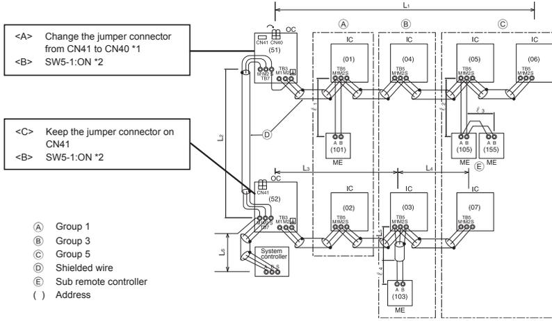
\*1 : When the power supply unit is not connected to the transmission line for centralized control, disconnect the male power supply connector (CN41) from ONE outdoor unit in the system and connect it to CN40 (except TKMU model). When the System controller is connected to TB7 side and TKMU outdoor unit model is used, connect a PAC-SC51KUA to TB7 side. If a PAC-SC51KUA cannot be used, connect the System controller to TB3 side. Up to three System controllers can be connected to TB3 side.
