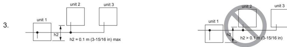
The NG example shows that oil accumulates into unit 1 while unit 3 is in operation, and unit 1 is stopped. Difference between unit and unit in height (h2) should be 0.1 m (3-15/16 in) or below.
