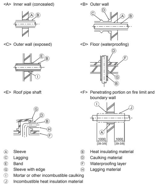
When filling a gap with mortar, cover the penetration part with steel plate so that the insulation material will not be caved in. For this part, use incombustible materials for both insulation and covering. (Vinyl covering should not be used.)
