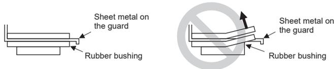
\*3 When tying the supplied tie band around the rubber bushing, make sure to leave no gap between the ends.
