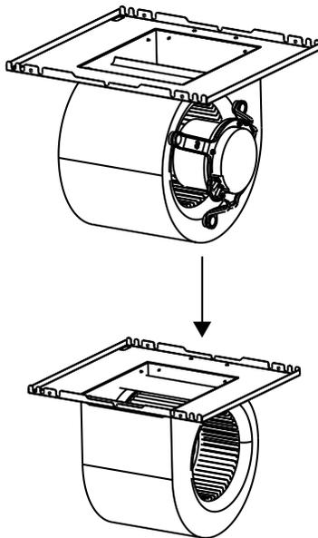
**Step. 6** Rotate the blower assembly 180°. The motor should now be on the opposite side.
