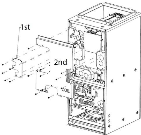
**Step. 3a** Remove the screws securing the (3) panels to the COIL panel shown in the image above. Remove the “1st” panel and “2nd” panel marked “COIL”.
