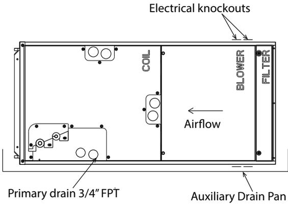
support the weight of the unit and connected ductwork. Vibration isolation is recommended for horizontal installations. Some jurisdictions may require an auxiliary drain pan be mounted under the unit. Always follow local or national code requirements.
