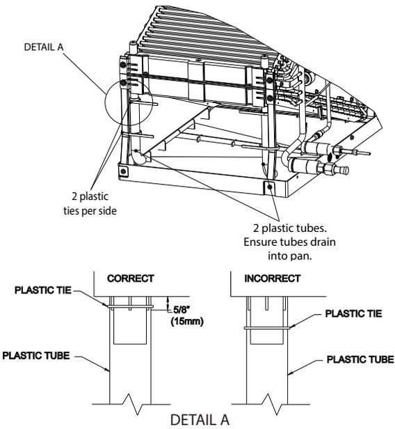
**Step. 10d** Next, install the clear plastic tubes which are included in the accessory bag. Ensure the plastic tubes drain into the pan. Also, be sure the clear plastic tubes do not have any restriction. Cutting of the plastic tube is required, please refer to the table below for length. Finally, secure the clear plastic tubes to the top drain pan per Detail A (see next page) then to the metal brackets supporting the coil to the top drain pan with the provided plastic ties as shown.
