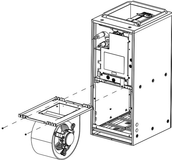
**Step. 5** Remove the (2) screws indicated in the image and slide the entire fan assembly out from the cabinet.
