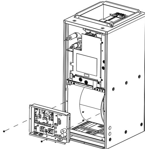
**Step. 4** Remove all electrical connections entering the control box. This includes the motor connector. Pull these harnesses from the control box. Next, remove the (2) screws indicated in the image and remove the control box from the air handler.
