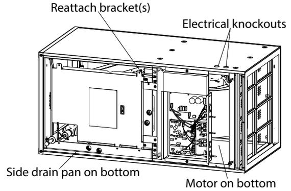
**Step. 11** Reinstall the coil assembly along with the bracket(s) that secure(s) it. Failure to reinstall the brackets will result in capacity loss and condensation formation inside the cabinet. Be sure the thermistor harness is reconnected inside the coil portion of the cabinet. Refer to 9.3 steps 1 to 4 to reassemble the panels. Ensure the proper knockouts are removed for drainage and electrical connections.
