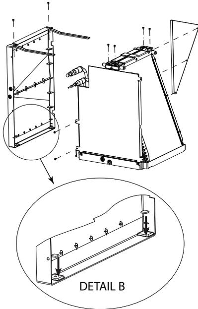
**Step. 10a** Install the (2) drain pan seals included in the accessory bag as shown in Detail B. These seals will cover the unused holes in the side drain pan to prevent leaks.
