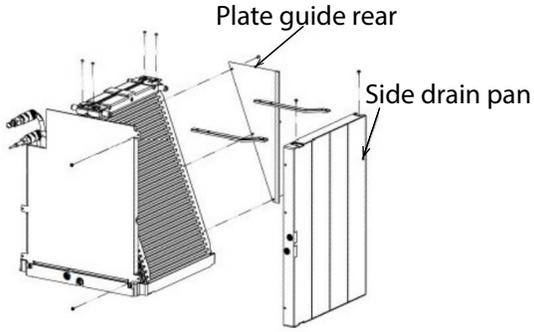
**Step. 9** Remove the Plate Guide Rear (3 screws) and Side Drain Pan (4 screws) along with supporting brackets (4 screws) from the coil assembly.
