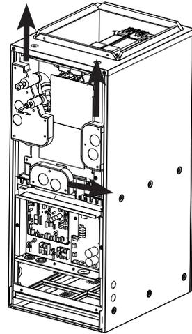
**Step. 3b** Next, remove the smaller panels covering the drain holes and refrigerant lines by first sliding in the direction indicated above.
