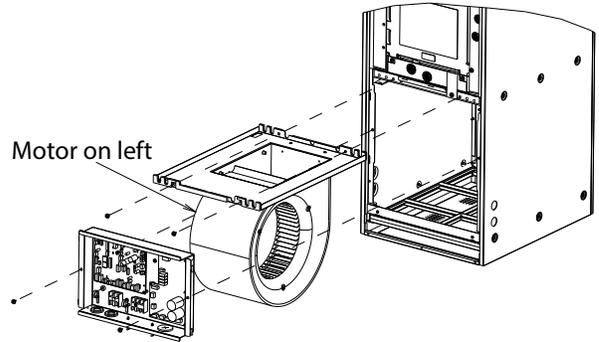
**Step. 7** Reinsert the blower assembly with the motor now on the left into the air handler cabinet and reuse the (2) screws that secured the fan assembly in position. Reroute the connector for the motor back into the enclosure and reconnect. Reinstall Control Box.
