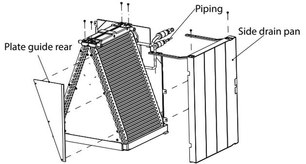
**Step. 10b** Reinstall the brackets to the opposite side of the Side Drain Pan. The Side Drain Pan will be reinstalled on the opposite side of the Coil Assembly. Reattach the Plate Guide Rear on the opposite side of the coil assembly.
