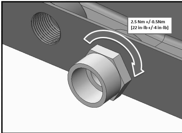
The air handler contains  $\frac{3}{4}$ " FPT drain connections. When the unit is used in the vertical position, there is one set. When the unit is mounted horizontally there is one set. Each set contains a primary drain and a secondary or auxiliary drain. The primary drain is the one that is lowest (even with the bottom of the pan). The secondary drain is at the higher level. They are labeled on the dimensional drawings above.
