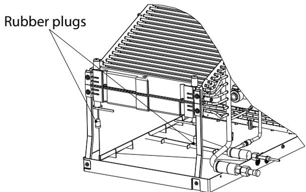
**Step. 10c** Remove the plugs indicated in the image above.
