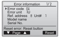
Error code, error unit, refrigerant address, unit model name, and serial number will appear.
