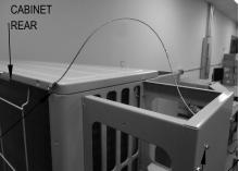
2 screws on the Front Panel connected to the Safety Cable-
