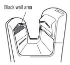
Sensor's sensitivity may be reduced if the black wall area is fouled in white. Clean the area at least once a week according to the Maintenance and cleaning of the exteriors.
