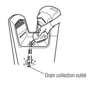
Pour 200ml (around 1 cup) of water through the drain hole. (To prevent it from getting clogged.)
