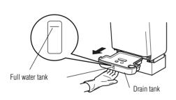
Pull the drain tank out horizontally.
