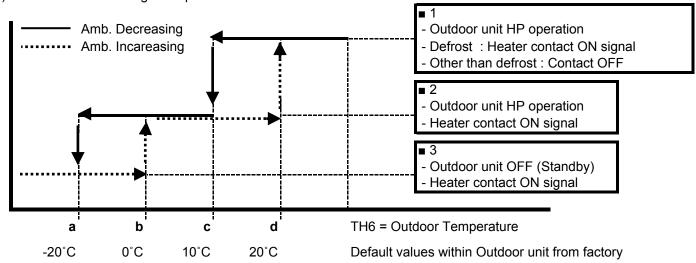
When the set temperature ranges overlap, the previously set pattern (1,2 or 3) has a priority. At default, the pattern 1 has the highest priority, 2 the second and then 3.
