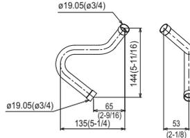
Note 1. Refer to the figure below for the installation position of the high-pressure twining pipe.
