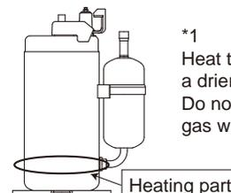
\*1 Heat the compressor with a drier for about 20 minutes. Do not recover refrigerant gas while heating.
