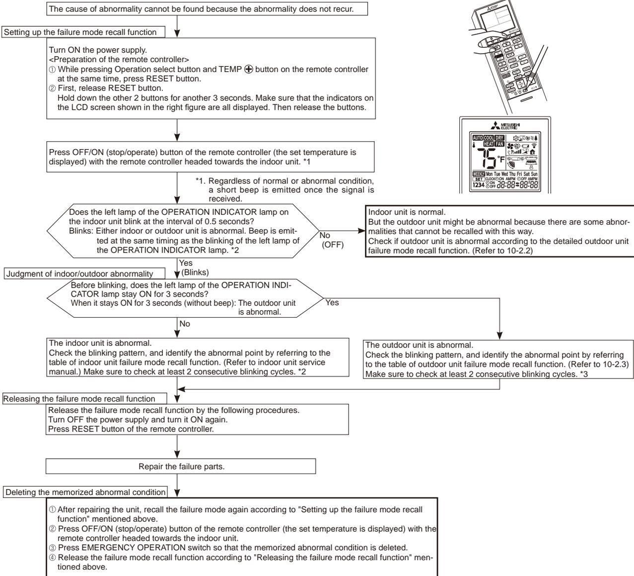
**NOTE:** 1. Make sure to release the failure mode recall function after it is set up, otherwise the unit cannot operate properly.
