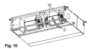
3. Removing the motor cable
