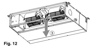
(4) Remove the four fan case fixing screws to take the top half of the fan casing off.
