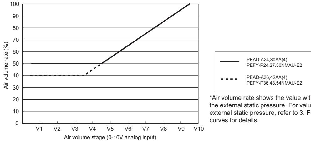
\*Air volume rate shows the value without change in the external static pressure. For values in different external static pressure, refer to 3. Fan characteristic curves for details.
