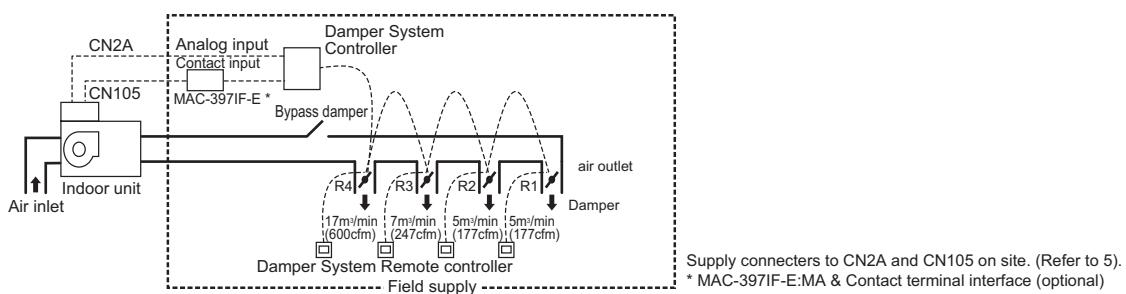
Check air volume at each air outlet when R1-R4 is full open and set static pressure as target value. Then, analog input to keep the static pressure at this target value even when either of the damper closes.
