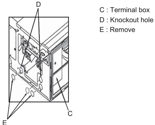
(3) Run wiring CN105 and CN2A through a knockout hole.
