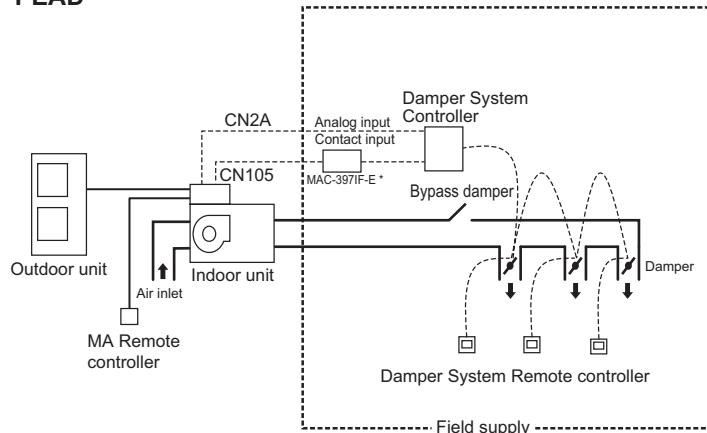
Supply connectors to CN2A and CN105 on site. (Refer to 5)
