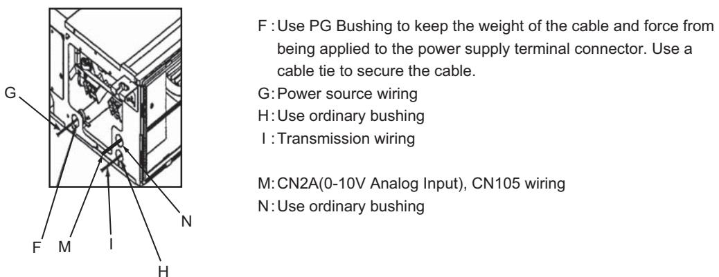
(4) Plug in connector CN105 (red) and CN2A (black) to the indoor controller board. Supply connectors to CN2A and CN105 on site.
