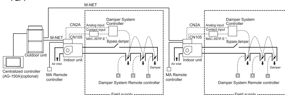
Supply connectors to CN2A and CN105 on site.
