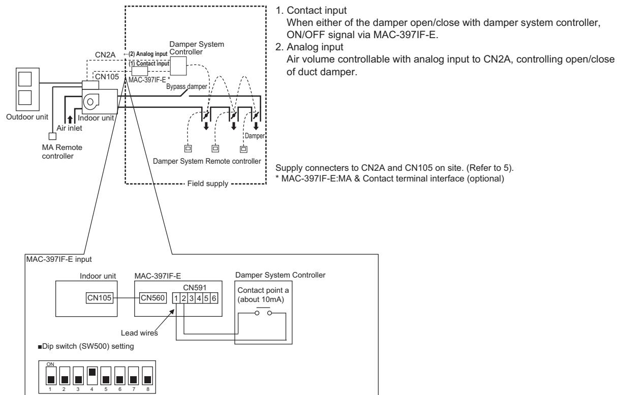
Refer to the MAC-397IF-E manual for DIP-SW setting and wiring.
