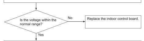
Check the fan motor position thermistor signal.
