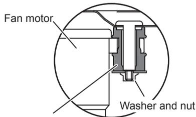
Note: When re-attaching the motor mount, make sure that the thicker end faces the motor shaft.
