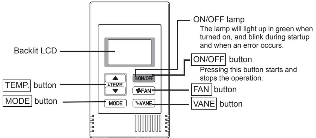
Note: To set the functions that are not available on this controller (PAC-YT53CRAU) such as Louver, use the centralized controller.
