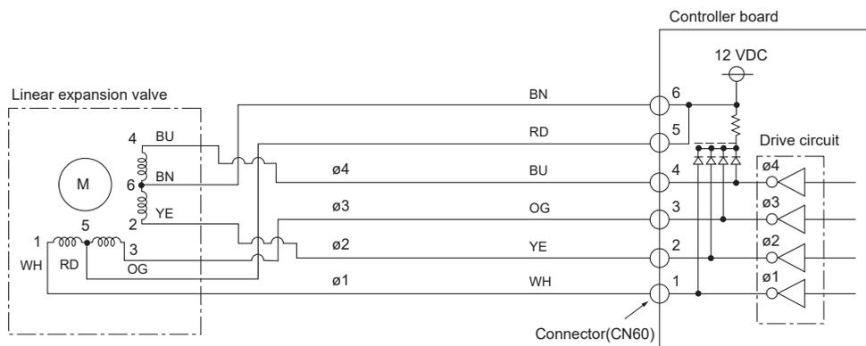
Note : Since the number of the connector at the controller board side and the relay connector are different, follow the color of the lead wire.
