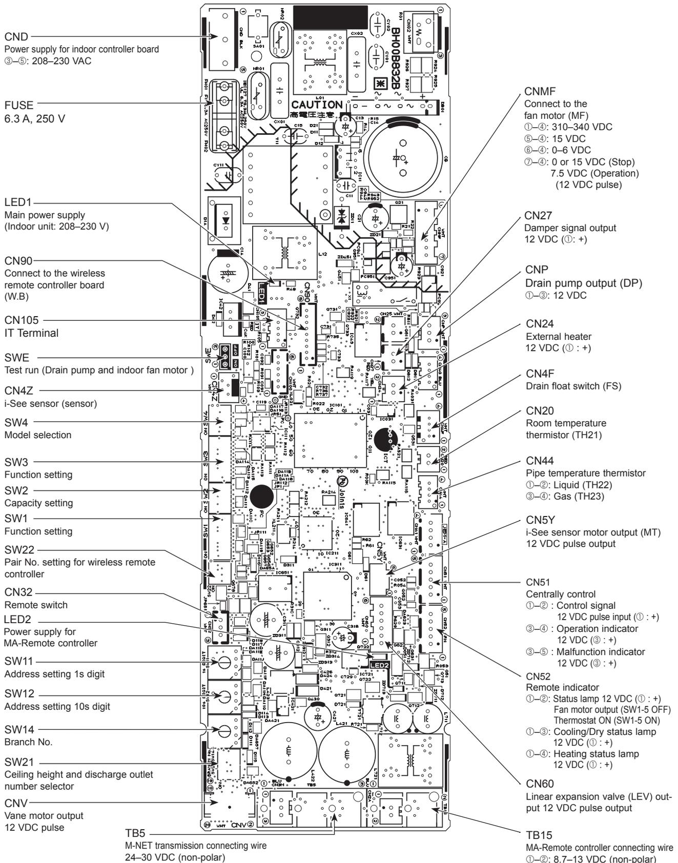
Note: The voltage range of 12 VDC in this page is between 11.5 to 13.7 VDC.
