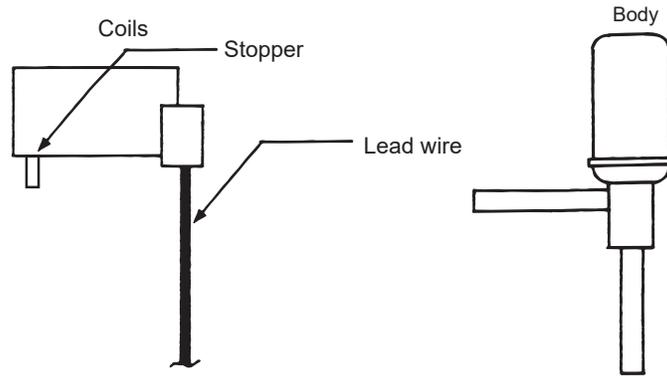
2) Removing the coils
