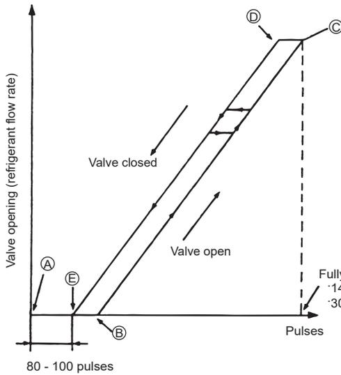
\*When the power is turned on, the valve closing signal of 2200 pulses will be output from the indoor board to LEV to fix the valve position. It must be fixed at point (A)
