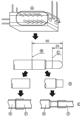
Be sure to have pipe expansion of indoor unit connecting port by cutting the piping at the cutting point which depends on the indoor unit capacity.
