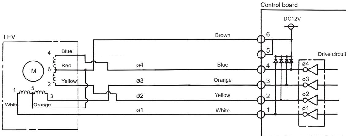
3) Pulse signal output and valve operation
