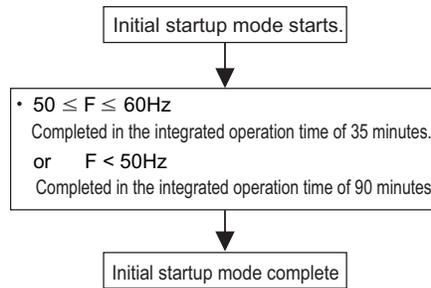
**(2) System with two heat-source units**
