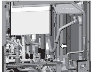
5) To remove the water heat exchanger
