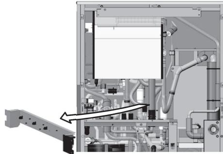
3) To remove the Water Heat Exchanger and Front Panel
