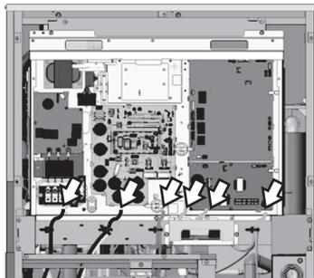
④ Remove the pipe cover and cable tie (total 3 places), and then disconnect the wire and sensor (TH7, TH8).
