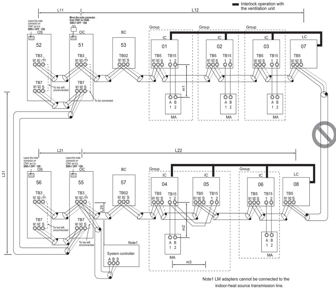
Note1 LM adapters cannot be connected to the indoor-heat source transmission line.
