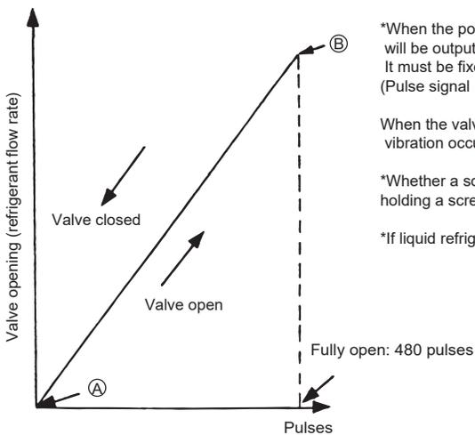
\*When the power is turned on, the valve closing signal of 520 pulses will be output from the indoor board to LEV to fix the valve position. It must be fixed at point (A) (Pulse signal is output for approximately 17 seconds.)
