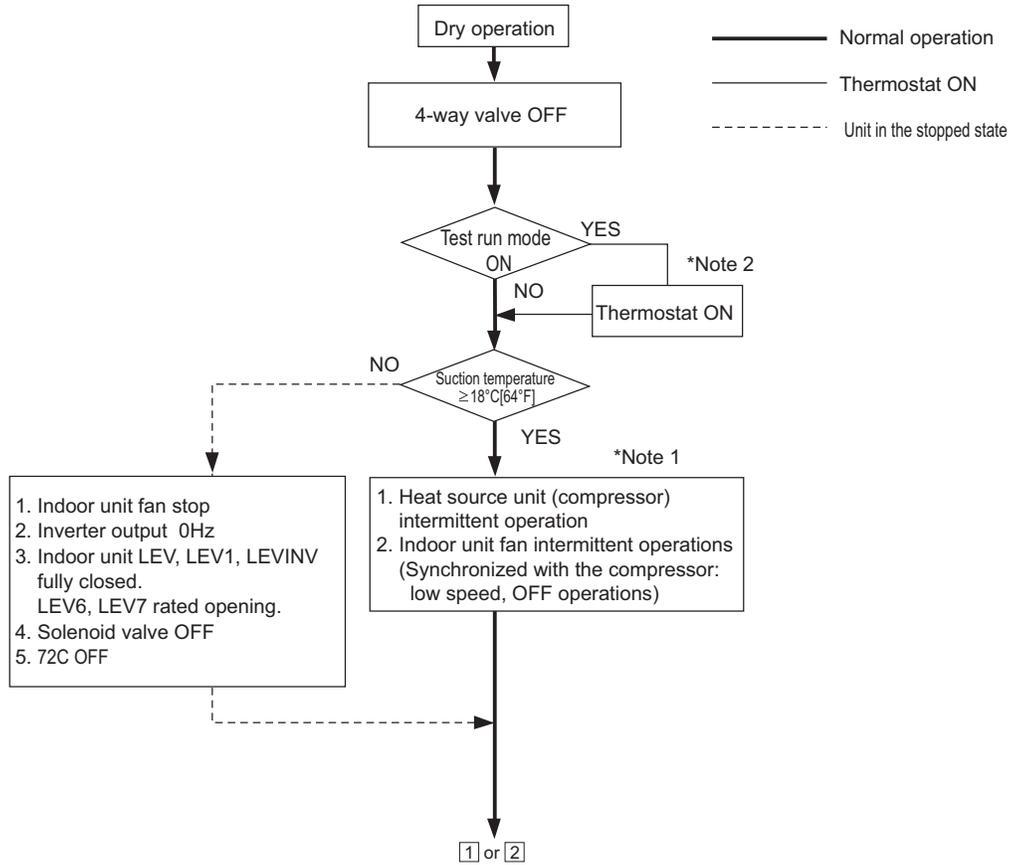
\*Note 1. When the indoor unit inlet temperature exceeds 18°C [64°F], the heat source unit (compressor) and the indoor unit fan start the intermittent operation simultaneously. When the indoor unit inlet temperature becomes 18°C [64°F], or less, the fan always runs (at low speed). The heat source unit, the indoor unit, and the solenoid valve operate in the same way as they do in the cooling operation when the compressor is turned on.
