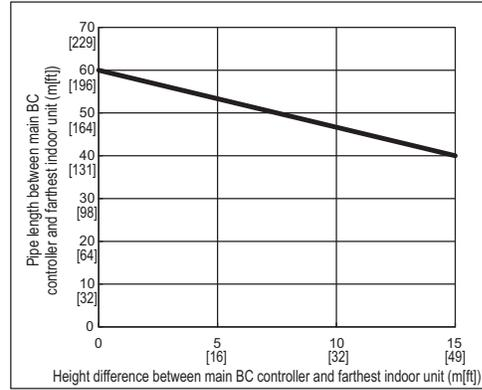
Piping length and height between IU and BC controller
