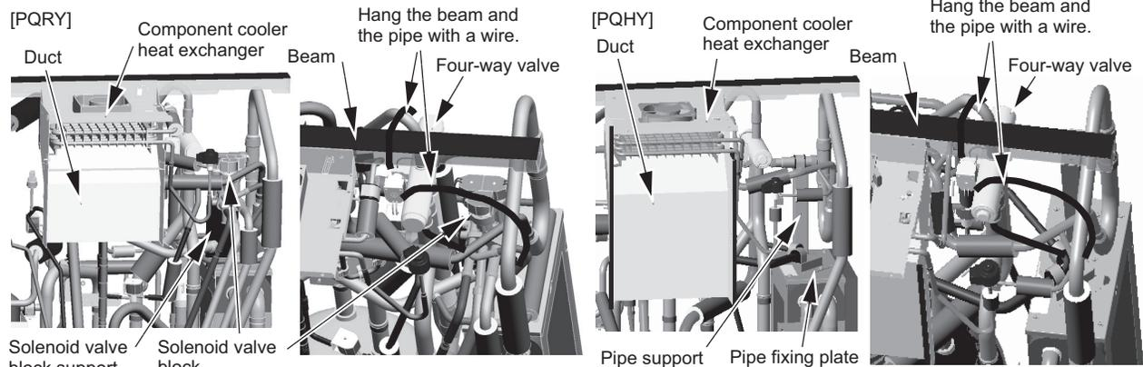
④ Unbraid the pipe, remove the pipe assembly (see the left figure below), and remove the water heat exchanger fixing screws.
