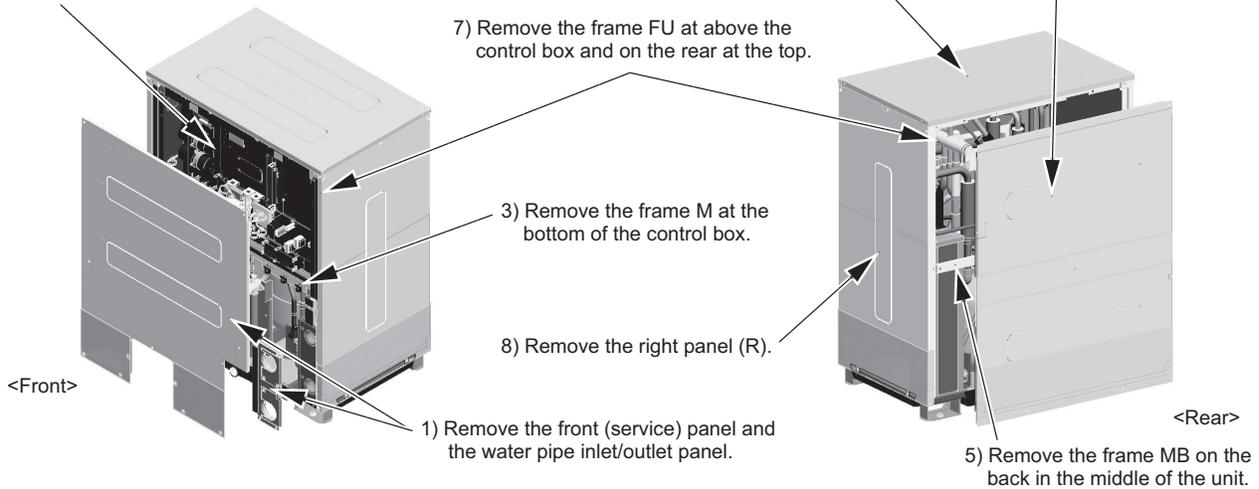
① After removing the right panel (R), hang the beam of the Component cooler heat exchanger from the four-way valve piping to keep the Component cooler heat exchanger from falling downward, using a wire (see the right figure below).
