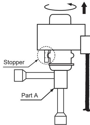
3) Installing the coil
