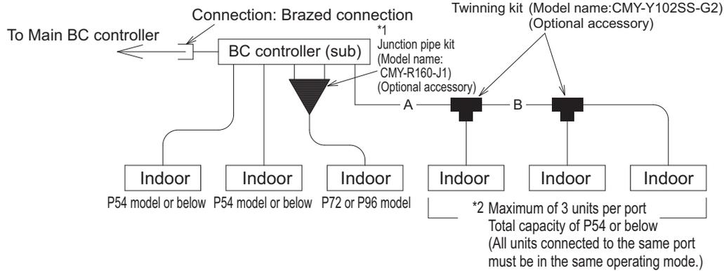
The ports of the BC controller accommodates the pipes on P54 model or below of indoor units. To connect other types of indoor units, follow the procedure below.
