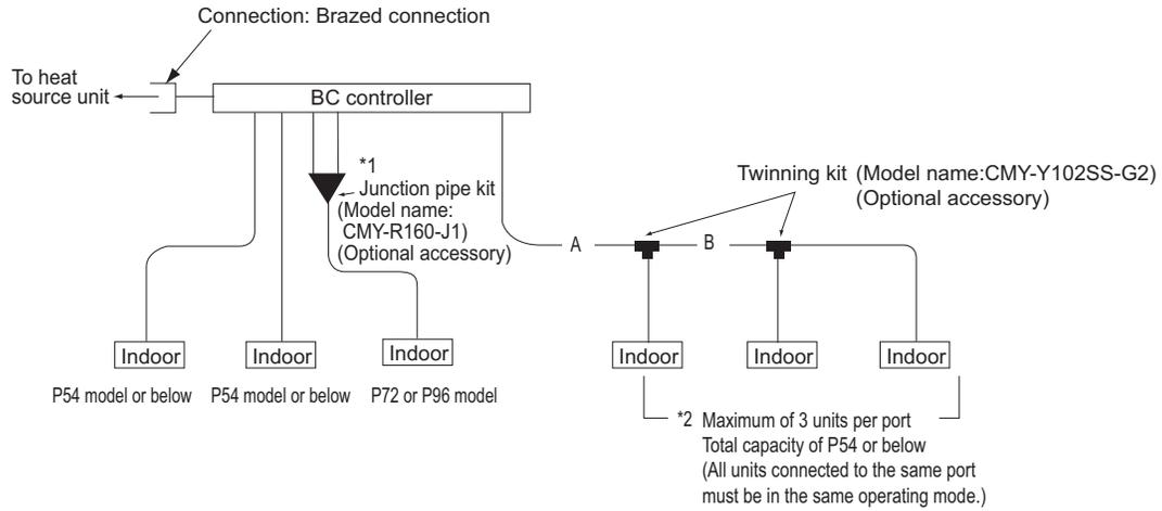
The ports of the BC controller accommodates the pipes on P54 model or below of indoor units.
