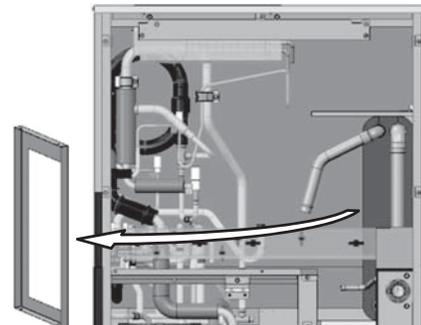
6) To move the Water Heat Exchanger
