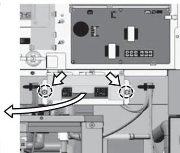
⑥ Remove the wire from cable strap on the Frame M.
