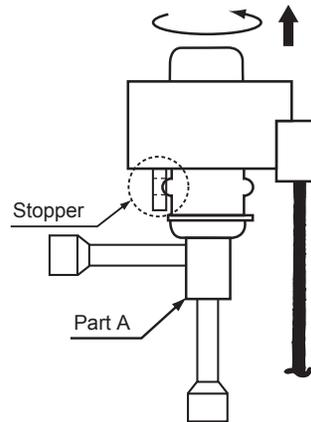
3) Installing the coil
