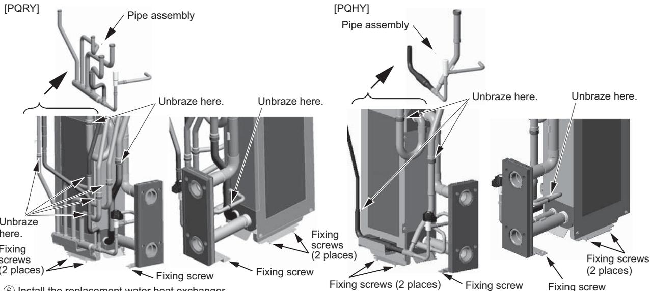
⑥ Install the replacement water heat exchanger.
