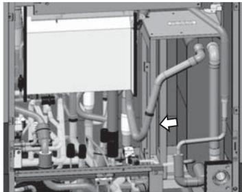
5) To remove the water heat exchanger
