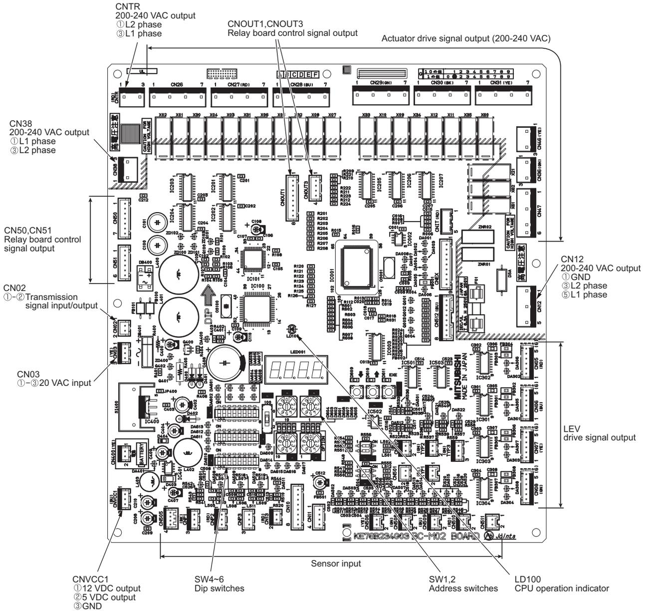
2. RELAY BOARD (RELAY 4 board)
