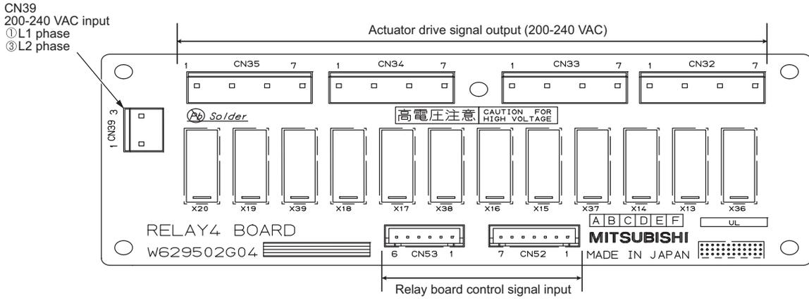
3. RELAY BOARD (RELAY 10 board)
