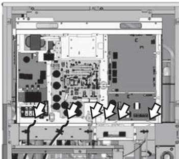
⑤ Remove the pipe cover and cable tie (total 3 places), and then disconnect the wire and sensor (TH7, TH8).
