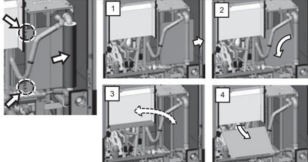
After removing Front Panel.
