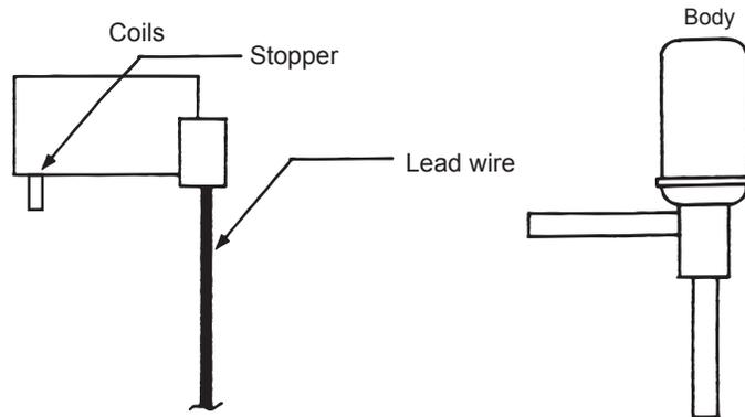
2) Removing the coils
