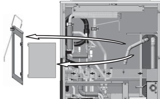
5) To remove the water pipe (2 pipes)
