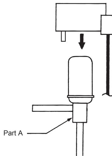
**(5) Heat source unit LEV (LEV6,LEV7) and BC controller coil removal procedure**
