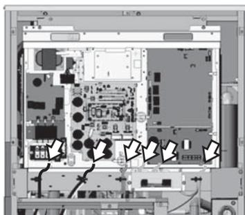
⑤ Remove the pipe cover and cable tie (total 3 places), and then disconnect the wire and sensor (TH7, TH8).
