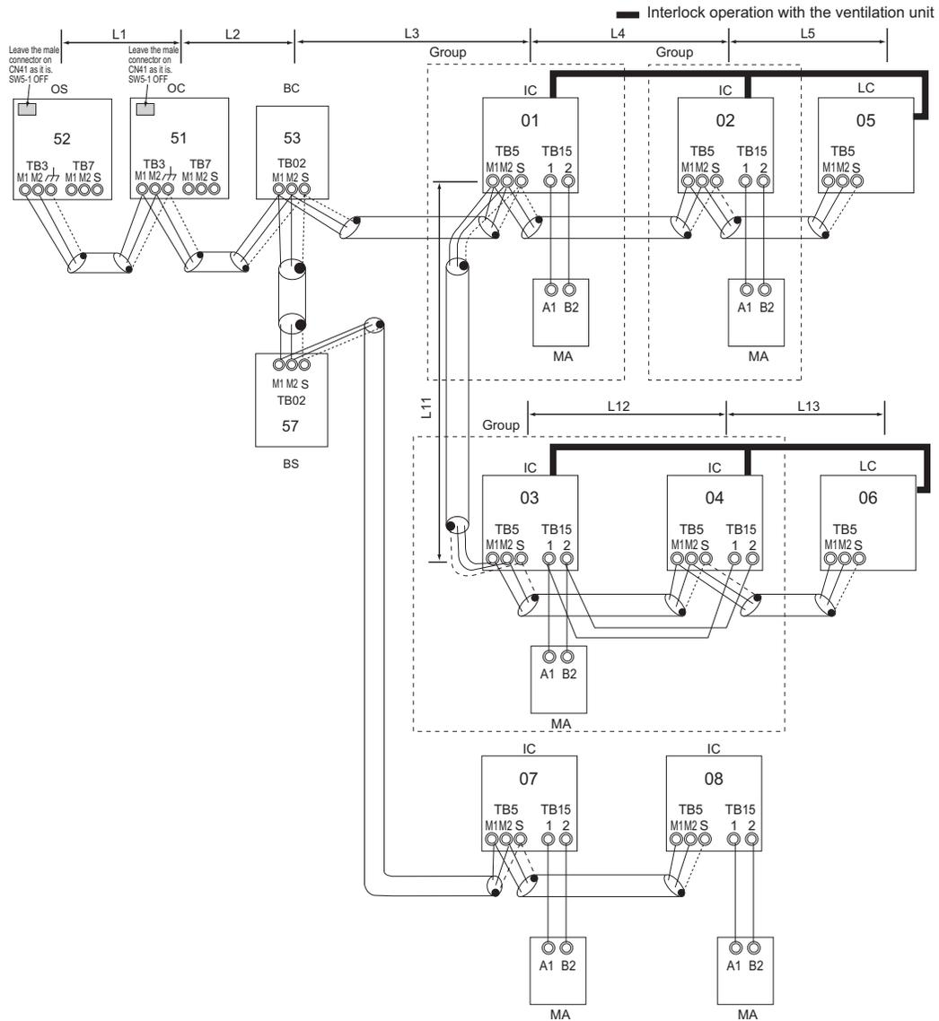
\* If the BC address overlaps any of the addresses that are assigned to either the OC, OS, or BS, use a different, unused address. OC, OS, and BS addresses (lowest indoor unit address in the group plus +50) have higher priority than the BS address.
