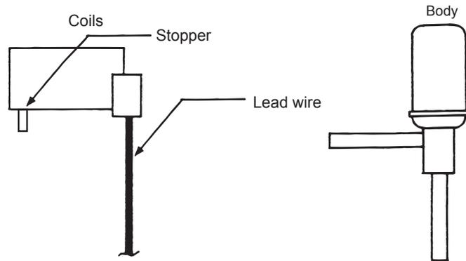
2) Removing the coils
