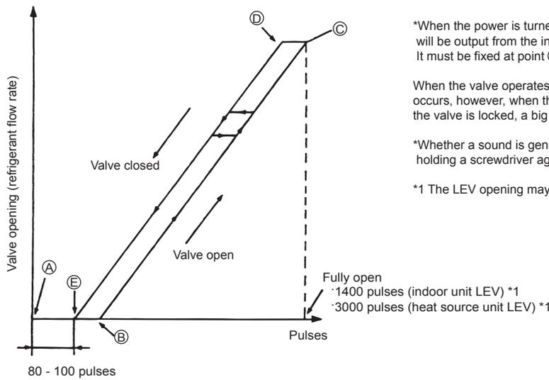
\*When the power is turned on, the valve closing signal of 2200 pulses will be output from the indoor board to LEV to fix the valve position. It must be fixed at point (A)
