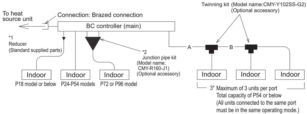
The ports of the BC controller accommodates the pipes on P24-P54 models of indoor units. To connect other types of indoor units, follow the procedure below.
