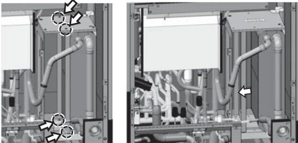
5) To remove the water heat exchanger
