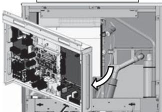
② Disconnect the wiring from the circuit board as shown in the figure.
