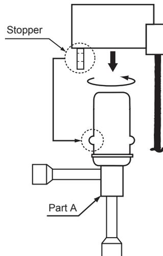
**(6) Indoor unit LEV, BC controller LEV coil removal procedure**
