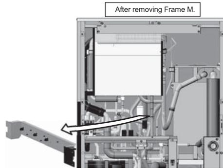
3) To remove the Water Heat Exchanger and Front Panel
