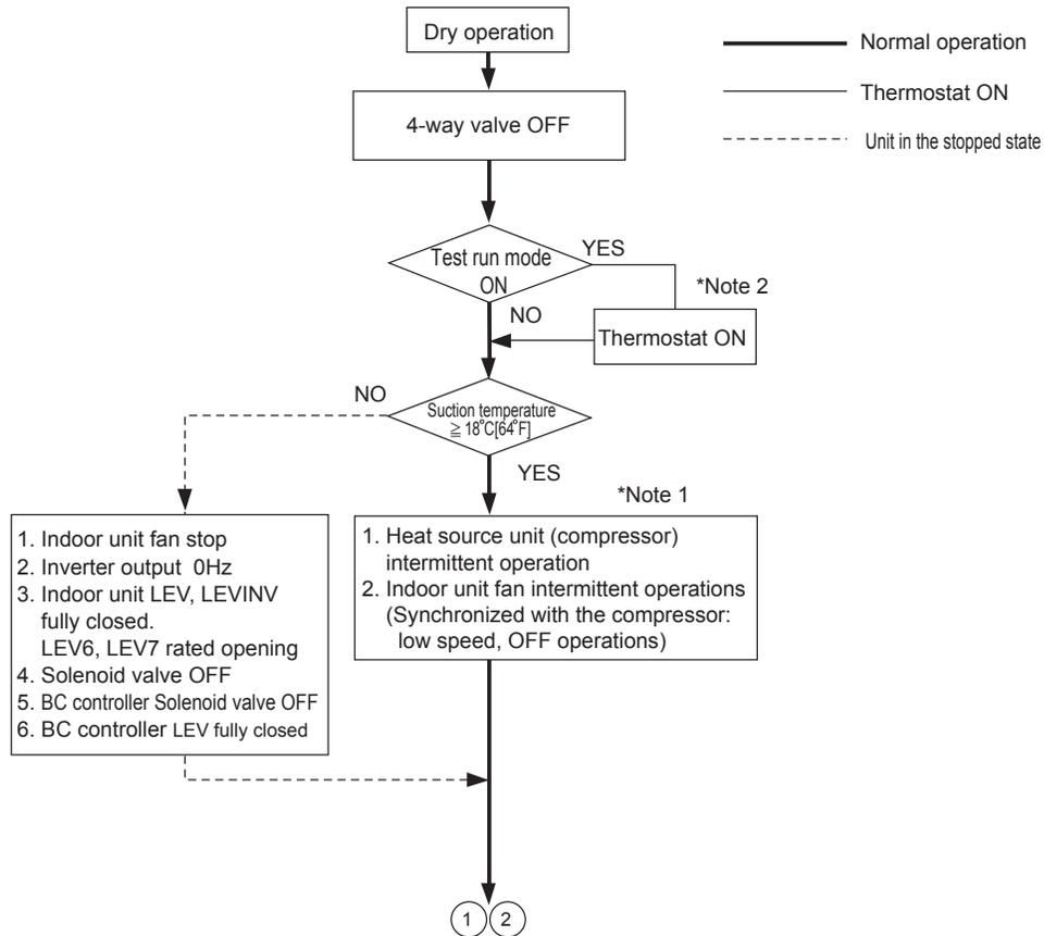
\*Note 1. When the indoor unit inlet temperature exceeds 18°C [64°F], the heat source unit (compressor) and the indoor unit fan start the intermittent operation simultaneously. When the indoor unit inlet temperature becomes 18°C [64°F], or less, the fan always runs (at low speed). The heat source unit, the indoor unit, and the solenoid valve operate in the same way as they do in the cooling operation when the compressor is turned on.
