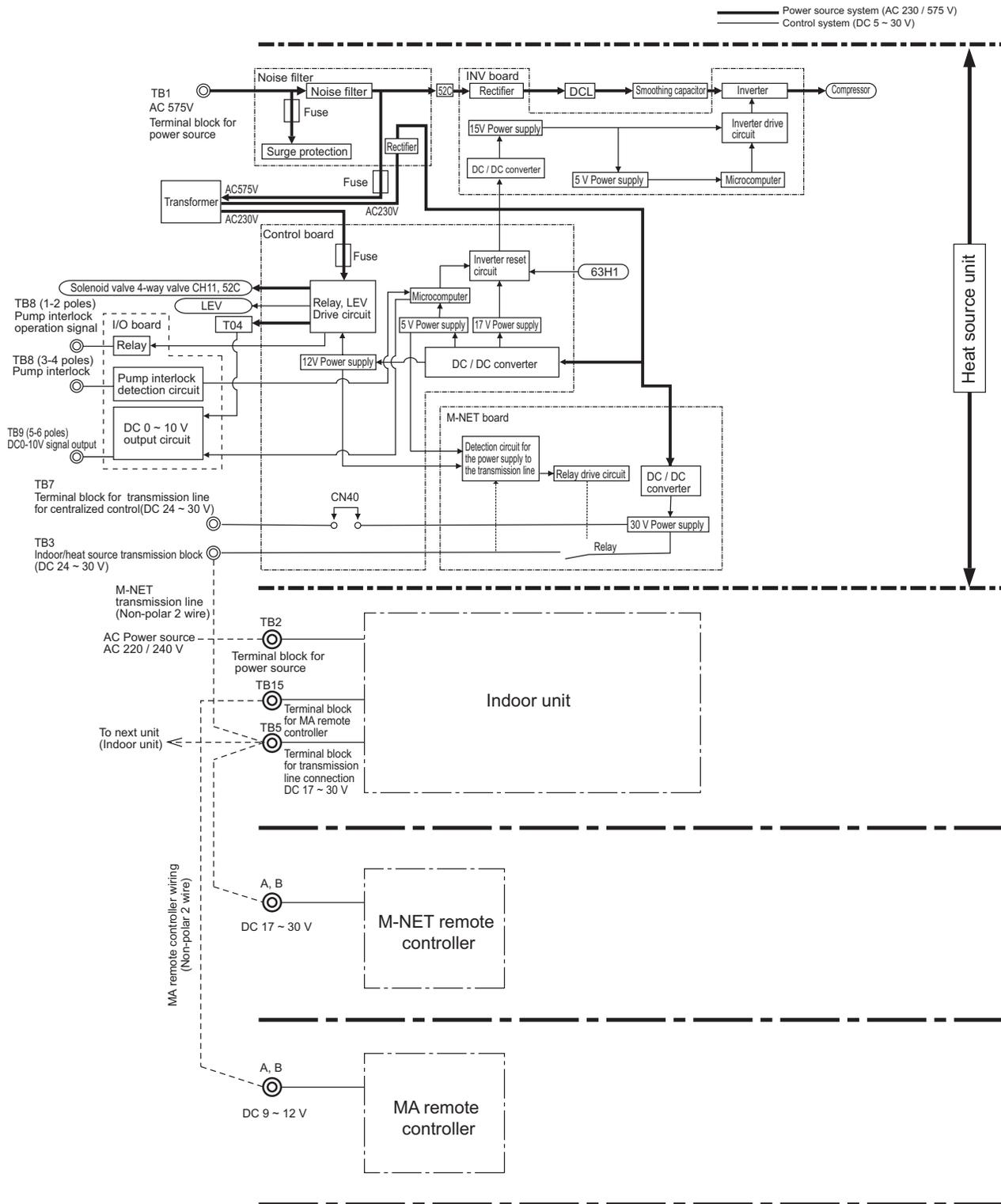
\* MA remote controllers and M-NET remote controllers cannot be used together.
