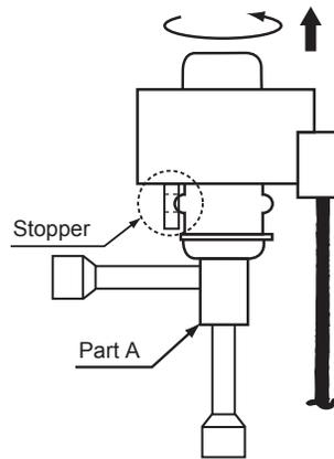
3) Installing the coil
