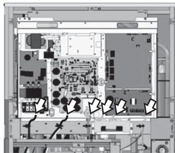
④ Remove the pipe cover and cable tie (total 3 places), and then disconnect the wire and sensor (TH7, TH8).
