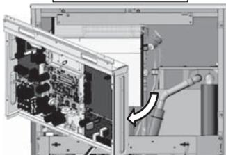
② Disconnect the wiring from the circuit board as shown in the figure.
