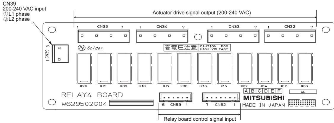
3. RELAY BOARD (RELAY 10 board)
