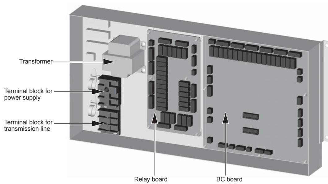
2. RELAY BOARD (RELAY 4 board)
