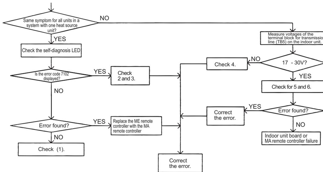
Refer to IX [4] -7- (2) "Troubleshooting transmission power circuit of heat source unit" for how to check item 1 in the flow chart above.
