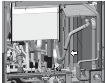
5) To remove the water heat exchanger
