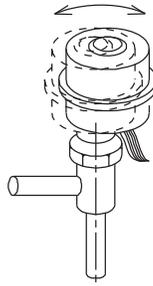
The motor may not be fixed with clamp because of the changing of the motor configuration. However, the fixing is not necessary due to the pipe fixing.
