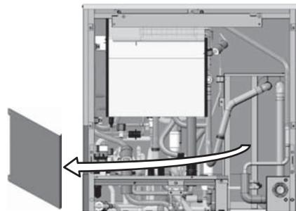
4) To move the Water Heat Exchanger and the Partition Plate
