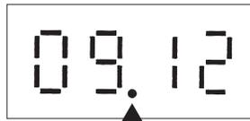
\* Disappears if the time data is deviated due to a power failure, or if a system controller that sets the time is not connected.
