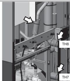
⑤ Remove the wire from cable strap on the Frame M.
