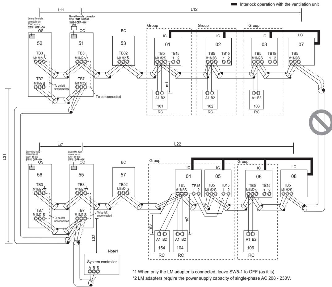
\*1 When only the LM adapter is connected, leave SW5-1 to OFF (as it is).
