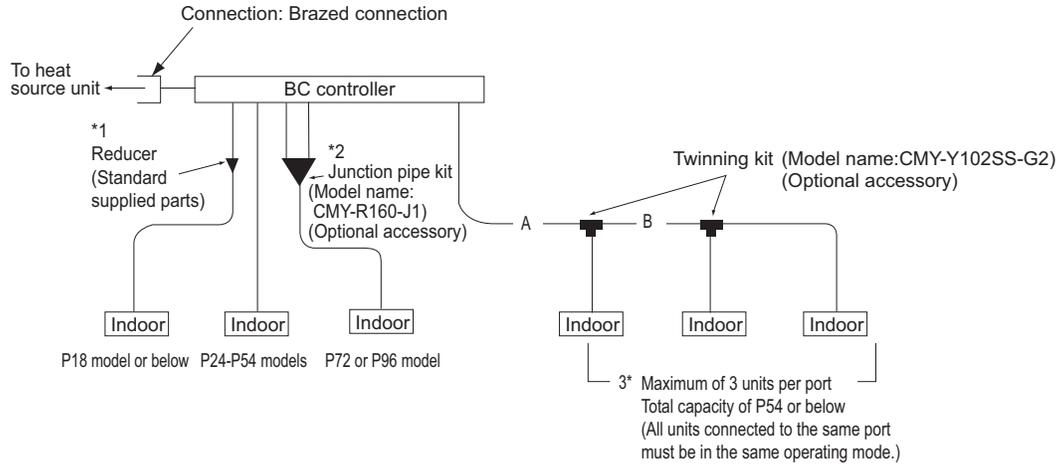
The ports of the BC controller accommodates the pipes on P24-P54 models of indoor units.
