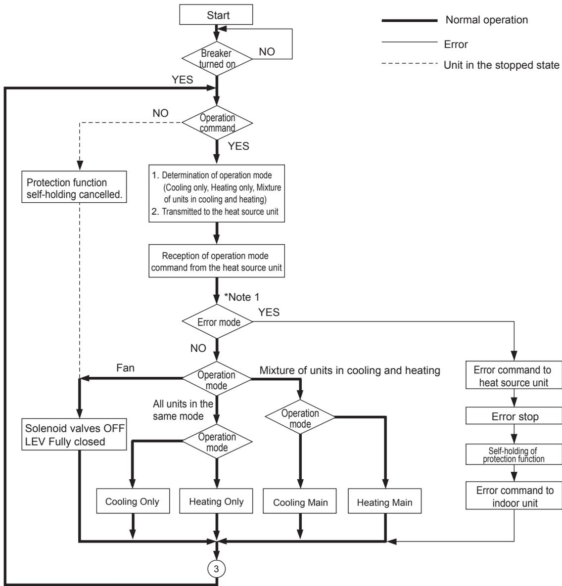
Note 1. The system may go into the error mode on either the indoor unit side or the BC controller or heat source unit side. If some of the indoor units are experiencing a problem, only those indoor units that are experiencing the problem will stop. If the BC controller or the heat source unit is experiencing a problem, all the connected units will stop.
