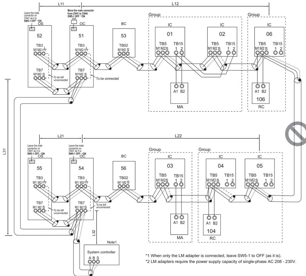
\*1 When only the LM adapter is connected, leave SW5-1 to OFF (as it is).
