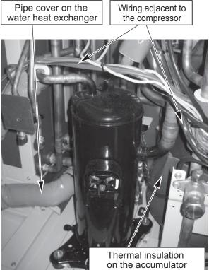
5. First, move the nearby wiring, insulation material on the accumulator, and pipe covers on the pipe and water heat exchanger out of the way or protect them from the brazing flame; then debraze the pipe, and replace the compressor.
