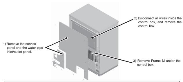
\* If the compressor is accessible by removing the rear service panel, it may facilitate compressor replacement.
