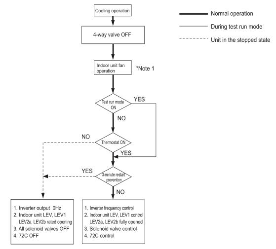
\*Note 1. The indoor fan operates at the set notch under cooling mode regardless of the ON/OFF state of the thermostat.
