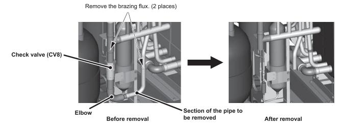
**%** The figures above are the views from behind to present a better view of the section to be removed.
