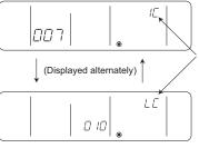
If registration is successfully completed, the two displays as shown on the left will appear alternately. If the registration fails, "88" will blink on the display.
