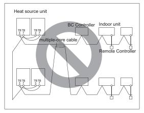
TB3: Terminal block for indoor-heat source transmission line TB7: Terminal block for centralized control
