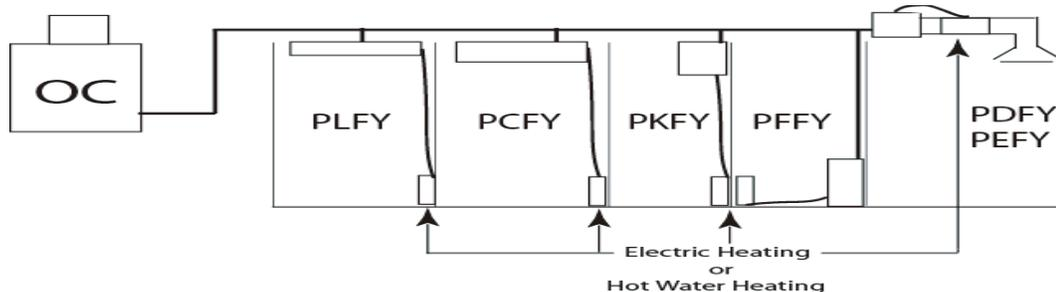
(2) Outdoor unit DIPSW4-4 for auxiliary heating control:
