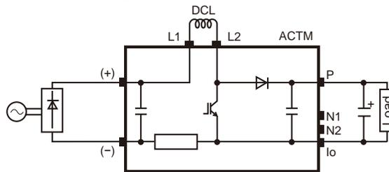
**Tester check points of Active filter module**
