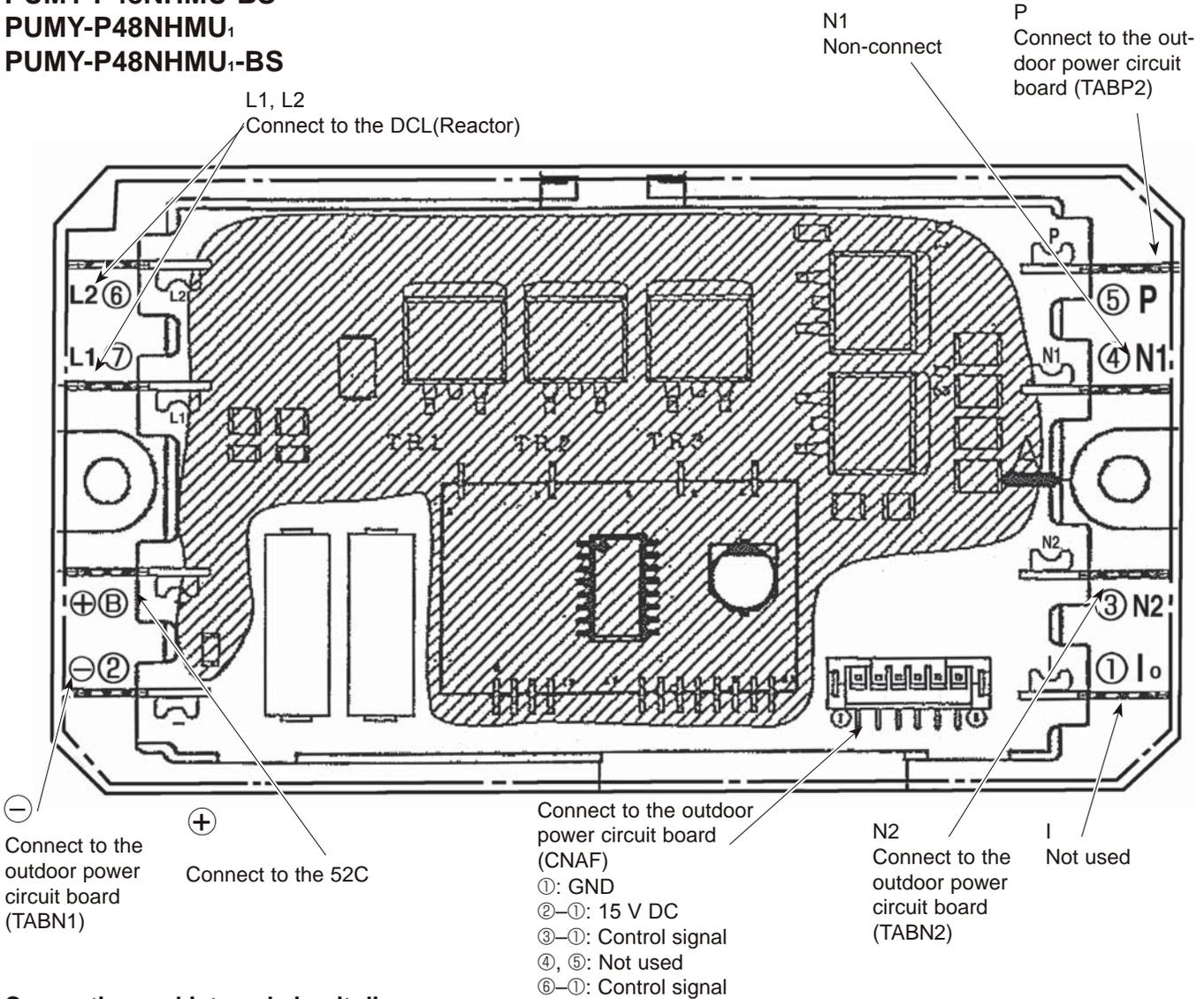
**Connection and internal circuit diagram**
