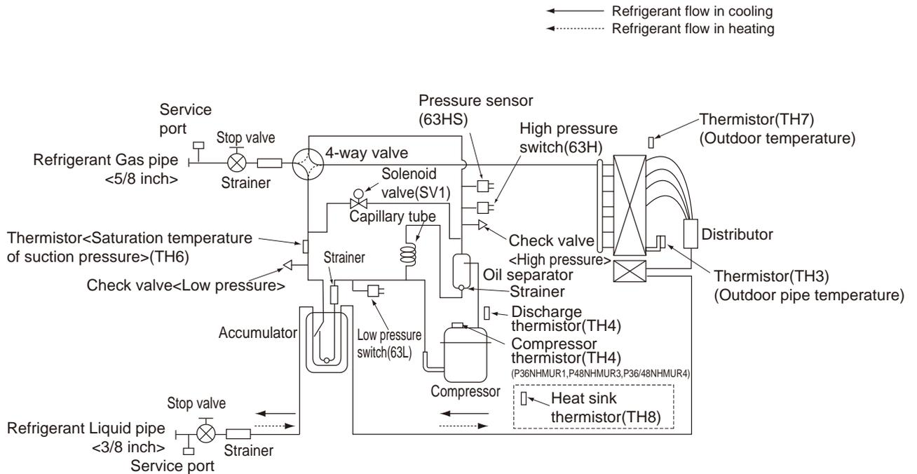
Capillary tube (for oil separator) :  $\phi(3/32) \times \phi(1/32) \times L(39-1/2)$  (in) [ $\phi 2.5 \times \phi 0.8 \times L1000$  (mm) ]
