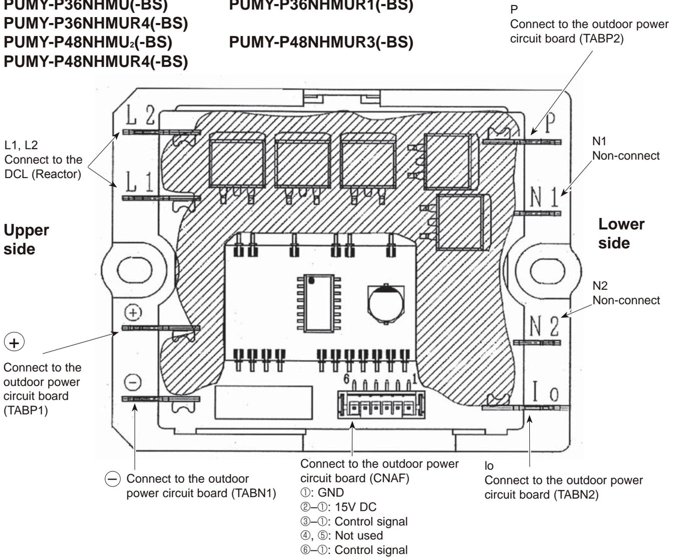
**Connection and internal circuit diagram**
