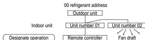
\* "88" will blink in the room temperature display area if the selected refrigerant address does not exist in the system. Furthermore, if "F" appears and blinks in the unit number display area and the refrigerant address display area also blinks, there are no units that correspond to the selected unit number. In this case, the refrigerant address and unit number may be incorrect, so repeat steps ② and ③ to set the correct ones.
