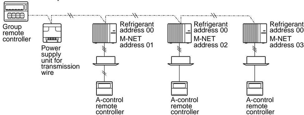
It would be ok if M-NET wire (non-polar, 2-cores) is arranged in addition to the wiring for A-control.
