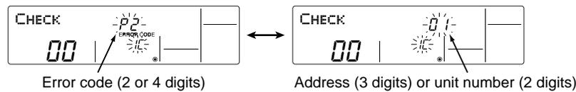
When using remote-/local-controller combined operation, cancel the error code after turning off remote operation. During central control by a MELANS controller, cancel the error code by pressing the **ON/OFF** button.
