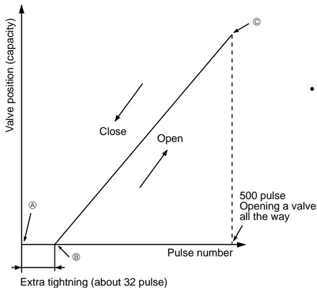
When the valve moves smoothly, there is no sound or vibration occurring from the linear expansion valve ; however, when the pulse number moves from ㉒ to ㉑ or when the valve is locked, sound can be heard.
