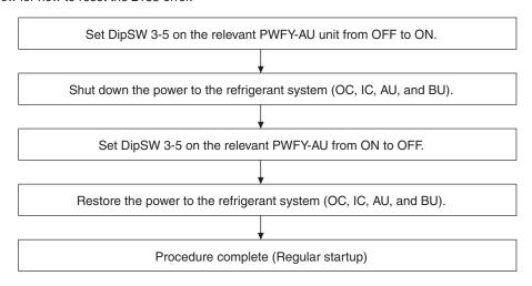
\* When a 2135 error occurs, the data before the error will be protected against overwriting. Set DipSW 1-8 of the relevant PWFY-AU unit from OFF to ON and then to OFF again to be disable the overwrite protection of 2135 error.
