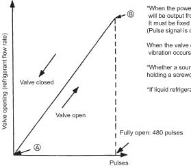
\*When the power is turned on, the valve closing signal of 520 pulses will be output from the indoor board to LEV to fix the valve position. It must be fixed at point (A).
