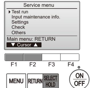
2. Select "Test run" with the [F1] or [F2] button, and press the [SELECT/HOLD] button.
