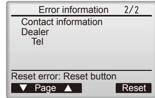
2. Press the **[F4]** button or the **[ON/OFF]** button to reset the error that is occurring.
