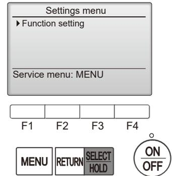
2. Set the indoor unit refrigerant addresses and unit numbers with the [F1] through [F4] buttons, and then press the [SELECT/HOLD] button to confirm the current setting.
