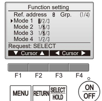
5. When the settings are completed, press the [SELECT/HOLD] button to send the setting data from the remote controller to the indoor units.
