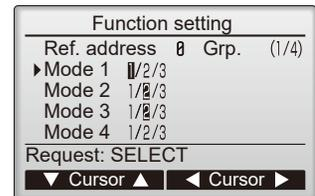
4. Use the [F1] or [F2] button to move the cursor to select the mode number, and change the setting number with the [F3] or [F4] button.
