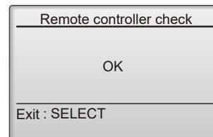
If the [SELECT/HOLD] button is pressed after the remote controller check results are displayed, remote controller check will end, and the remote controller will automatically reboot itself.
