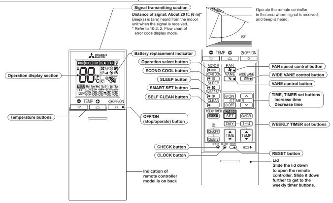
**NOTE**: Last setting will be stored after the unit is turned off with the remote controller. The indoor unit beeps when it receives the signal.
