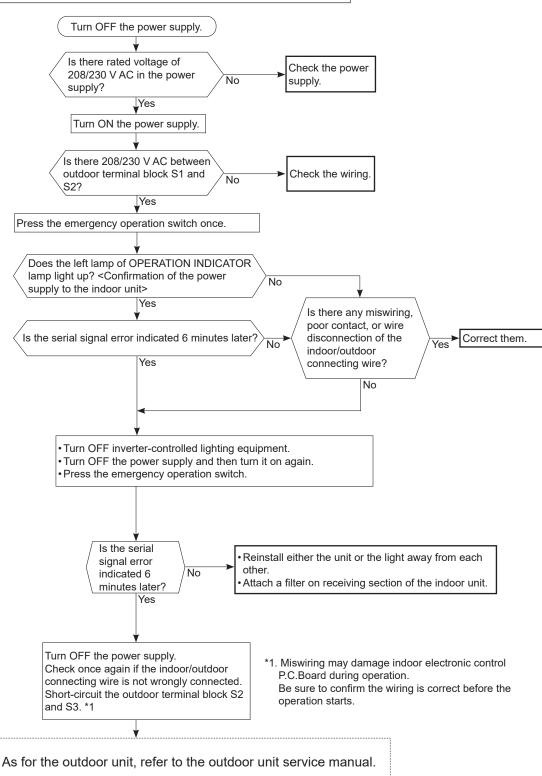
When the left lamp of OPERATION INDICATOR lamp blinks 9-time, the indoor unit and outdoor unit do not operate.
