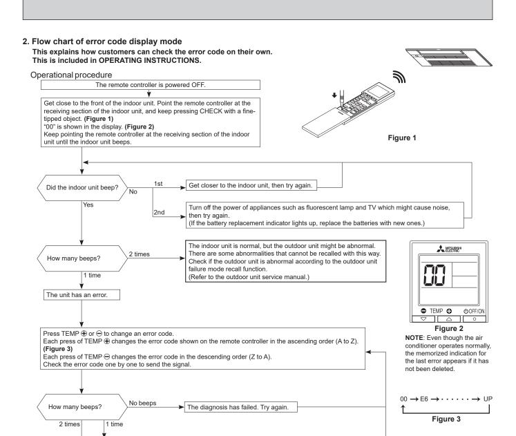
Refer to the error code on the table of the indoor unit failure mode recall function (10-2.3.) or the table of the outdoor unit failure mode recall function (refer to the outdoor unit service manual).
