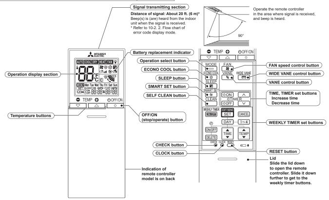
**NOTE**: Last setting will be saved after the unit is turned off with the remote controller. The indoor unit beeps when it receives the signal.
