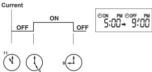
**NOTE:** If the main power is turned off or a power failure occurs while ON/OFF timer is activated, the timer setting is cancelled. As these models are equipped with an auto restart function, the air conditioner starts operating with timer cancelled when power is restored.
