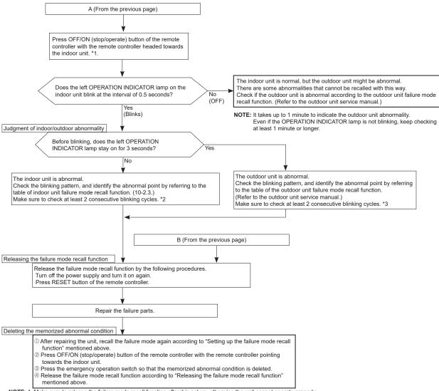
NOTE: 1. Make sure to release the failure mode recall function after it is set up, otherwise the unit cannot operate properly.2. If the abnormal condition is not deleted from the memory, the last abnormal condition is kept memorized.
