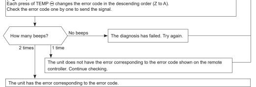
Refer to the error code on the table of the indoor unit failure mode recall function (10-2.3.) or the table of the outdoor unit failure mode recall function (refer to the outdoor unit service manual).
