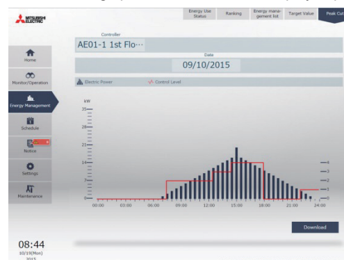
<Status of peak-cut control: Average power for 30 minutes, display of peak-cut control level>
